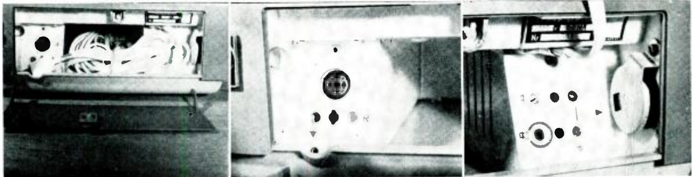
Removable door in side of case covers storage compartment and inputs and outputs. Left: cords and mike fit in center well. Center: PA amplifier switch is metal button at upper left of photo. Grouped on panel are microphone jack, radio-phono input jack and output jack for playing through separate amplifier. Right: other panel contains headphone jack, external jack and voltage adaptor (with small window).
