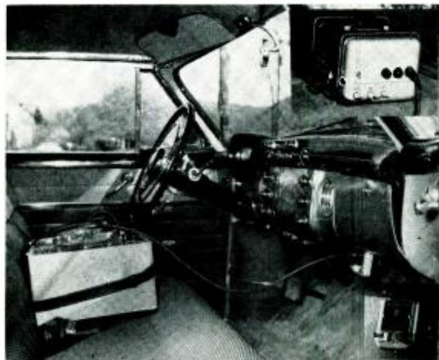
Any recorder may be used in the car if an inverter is used to provide 110 volts from the car battery. Insets show the ATR inverter mounted in the trunk and the small control panel for the dash. The recorder should be strapped to the seat to take care of sudden stops.
